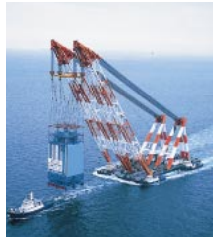
Desulfurization Plant Absorber Module for Electric Power Development Co., Ltd
